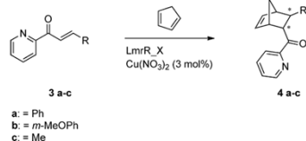
Scheme 1. Asymmetric Diels-Alder reaction catalyzed by LmrR_X/ Cu(NO 3 ) 2 complexes in a MOPS buffered solution.
